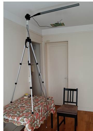
FIGURE 11. Nordic Semiconductor angle of arrival estimation test setup.
