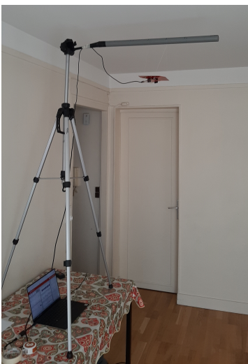
FIGURE 7. BOOSTXL-AOA angle of arrival estimation test setup.
