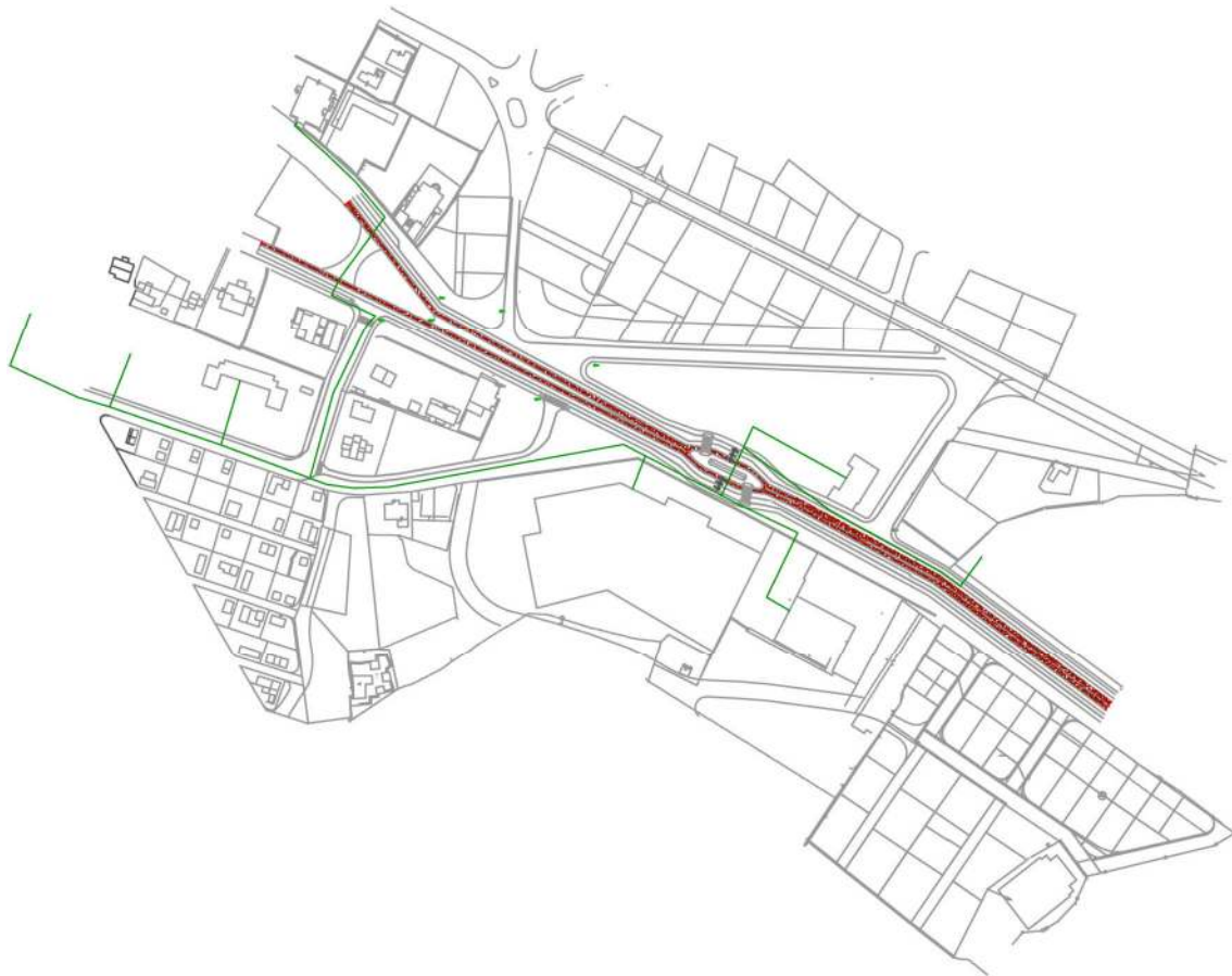
Fig. 8. Bus stop location and circulation scheme of the BRT system in Nablus
