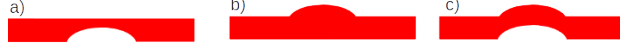
Figure 7: Different kinds of pixels detected as irregular: a) concave only irregularity, b) convex only irregularity, c) symmetric irregularity.
