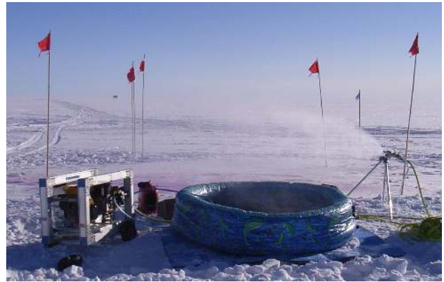
Figure 1. The production of the ^2\text{H} -labelled layer of snow at Summit, 8 August 2007. From left to right the air compressor/water pump rack, the inflatable water container and the snow gun.
