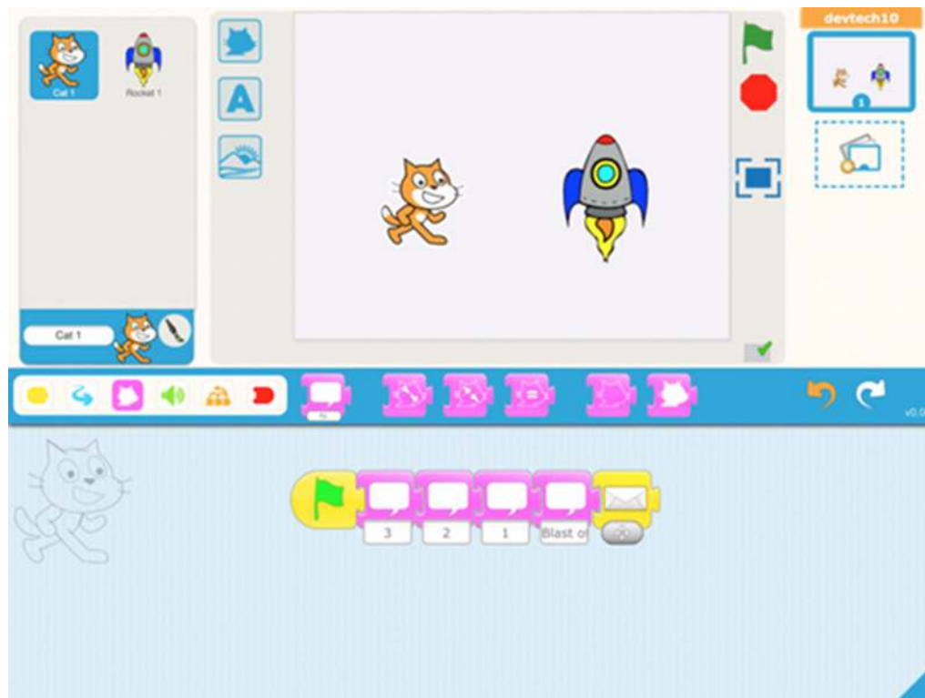
Fig. 3 ScratchJr project with Cat 1 script for counting down and “sending a message” to Rocket 1. (Color figure online)
