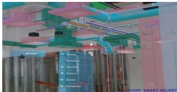
Figure 4 - Helmet vision with smart glasses: constructive details are shown, which are only in the design.
