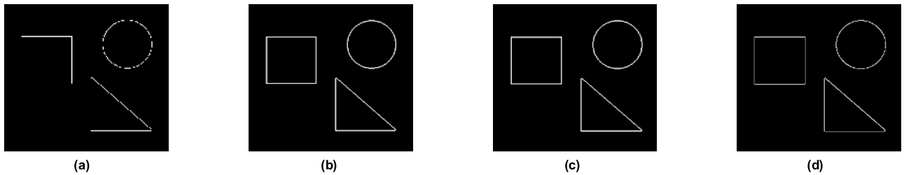
FIGURE 9. Results of border extraction by morphology difference operations with different structuring elements on simple binary image. (a) Borders extracted manually. (b) Result of morphological border extraction with cross-shaped structuring element. (c) Result of morphological border extraction with circular structuring element. (d) Result of morphological border extraction with proposed adaptive structuring element.
