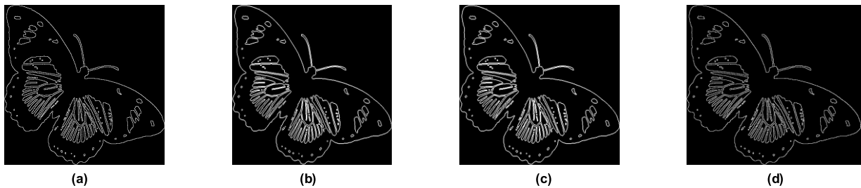
FIGURE 11. Results of border extraction by morphology difference operations with different structuring elements on complex binary image. (a) Borders extracted manually. (b) Result of morphological border extraction with cross-shaped structuring element. (c) Result of morphological border extraction with circular structuring element. (d) Result of morphological border extraction with proposed adaptive structuring element.
