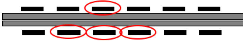
Figure 5-10: A schematic drawing of a module showing which chips overlap and so might have hits in coincidence due to the stereo-angle between the two sides of the module.
