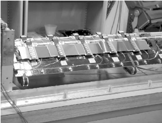
Fig. 18. Photograph of 10 barrel modules mounted on the carbon-fibre structure for system test.
