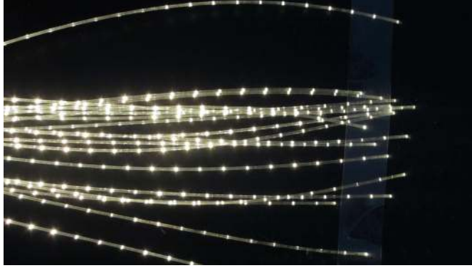
Figure 6: A bundle of clear fibres. Each fibre has 18 notches to supply the LED light to the 18 strips in a row of scintillators.
