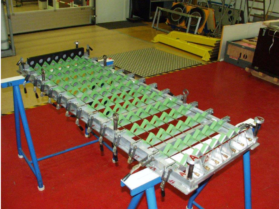
Fig. 16. Tooling used to produce a spacer.
