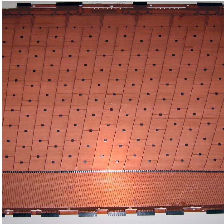
Fig. 7. Upper part: etched pattern, before folding, on A+B electrodes signal layer. Lower part: picture of a section, about 50 cm long, of an A electrode, before folding, showing the etched pattern of the HT layer where the resistive silk-screened pads of carbon-loaded epoxy ink can easily be seen. (The copper strips between connectors have not yet been removed.)
