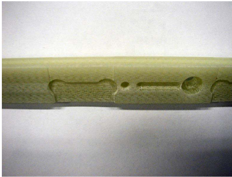
Fig. 4. G10 bar: transverse view drawing showing the 2\pi/1024 angle and picture of a bar section (10 cm long) showing holes for dowel pins and cut-outs for connectors.
