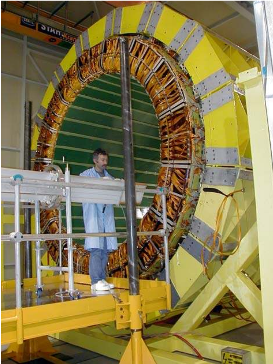
Fig. 31. Insertion of a barrel presampler sector.
