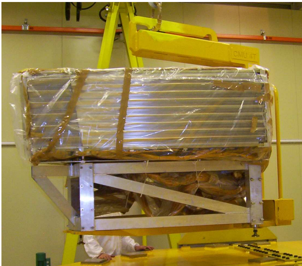
Figure 16. Positioning of a module on the assembly table. Observe the spatula and the lifting frame.
