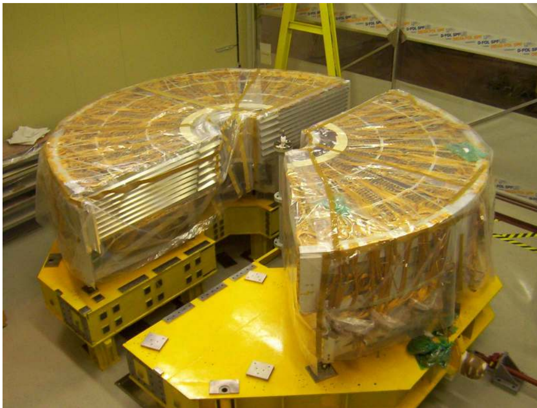
Figure 20. This picture shows the assembly table opened just before the installation of the last module. Observe the three reference plates on which the feet of the spatula of this last module will lay. The central axis is also visible.
