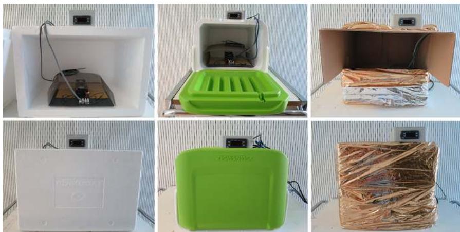
Figure 10: Incubator shells tested. Open (upper row) and closed (bottom row). Polystyrene foam box (left), thickness of 3.5 cm, outer dimensions 39 x 56 x 36 cm; hard plastic cooler box (middle), thickness of 2.5 cm, outer dimensions 32 x 41 x 47 cm; cardboard box (right) covered with a standard survival blanket of a thickness of 12 \mu m folded twice, outer dimensions 30 x 42 x 37 cm. Please click here to view a larger version of this figure.
