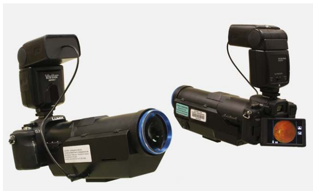
FIGURE 4. Front and rear depictions of the prototype low-cost fundus camera. The design uses a consumer camera for intuitive, point-and-shoot operation.
