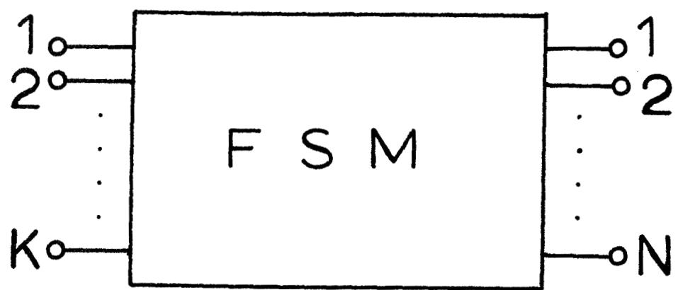
Fig. 1.1. An  $(N, K)$  general convolutional encoder.
