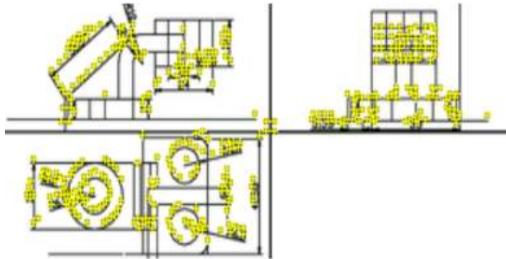
Fig. 3. Nature-feature points in a mechanical 2D drawing
