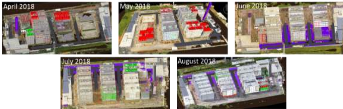
Figure 3: Visual models of progress (4D BIM + point cloud) with color codes
