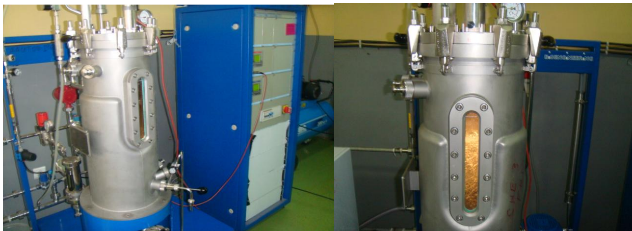
Figure 2. Fermenter (40l, Bioengineering, England, 2005)
