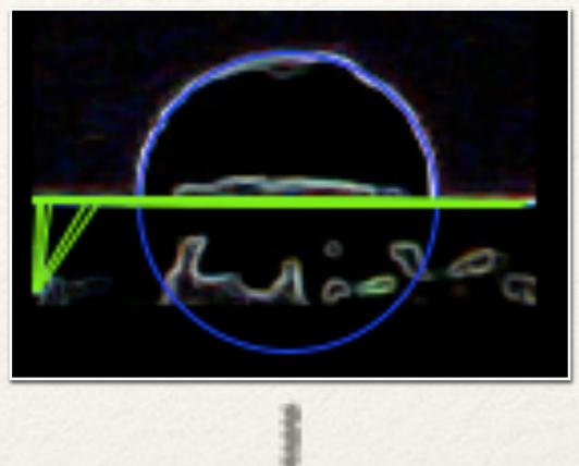
The geometry of the detected circle and surface is analyzed to determine the angle of contact between the two.
