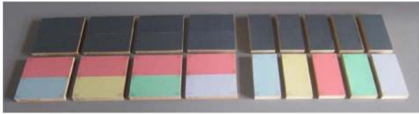
Figure 1. Stimuli. The stimuli were attached to wooden plates (50×100×12 mm). The sandpapers in the upper row belong to the rough group and the lower sandpapers belong to the smooth group. Left: in order for the participant to be able to quickly switch between stimuli, pairs of stimuli were prepared for the discrimination task. Different roughnesses have different colors in the smooth group. doi:10.1371/journal.pone.0093363.g001
