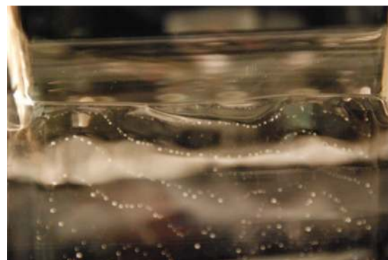
FIG. 10. Barring on the liquid film coated on the substrate at Q \sim 1.18 cm 2 /s and at U_w \sim 11 cm/s.
