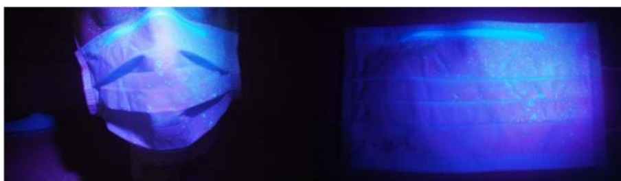
Fig. 2 Fluorescent particles (UV Glow powder) following spraying from 1 m from the side of the mask
