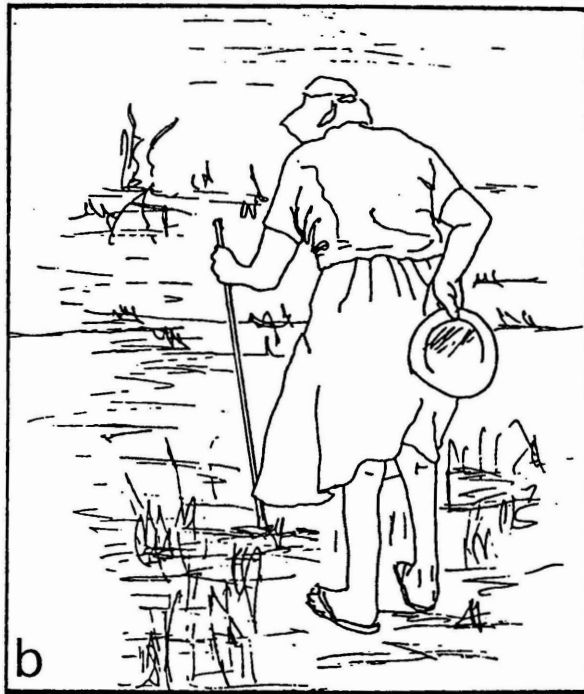
Figure 7.3: A crowbar used as a probe, (a) two-handed (b) one-handed.
