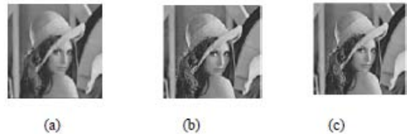
Figure 2: SPIHT results (a) Original image (b) levels of decomposition=3, 0.7 bpp (c) levels of decomposition= 9, 0.1 bpp
