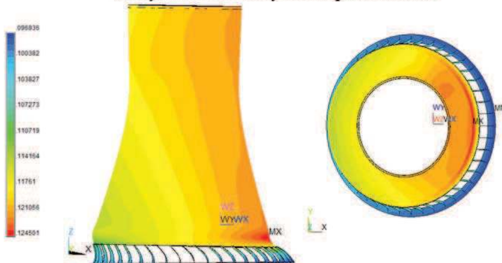
Total displacement (m) at the time t = 8.85 s. Structural analysis with allowance of accelerogram based on direct dynamic method
