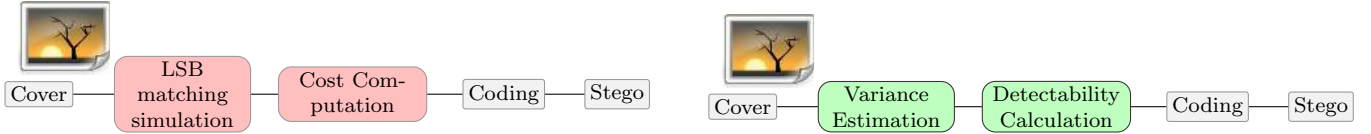
Figure 1. Simplified flowchart of a typical prior-art adaptive embedding scheme (left) and the proposed MiPOD (right).
