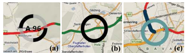
Figure 3: Polymodal navigation element: (a) Change to content-aware navigation is possible; (b) Indication of position along the road; (c) Indication of selection at a junction
