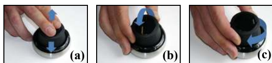
Figure 2 (a) Push/pull; (b) Tilting; (c) Rotation
