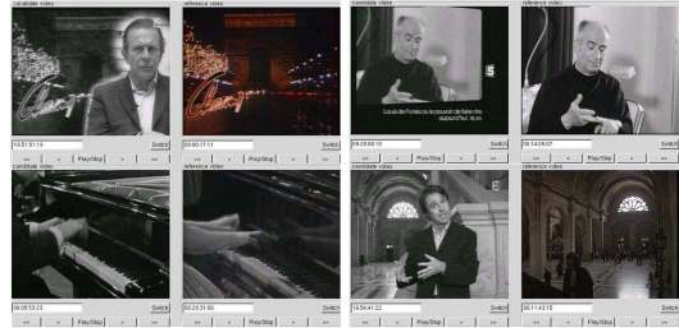
Fig. 17. Two good detections (up) and two false alarms (bottom) of the TV monitoring system: the left image of each match is the broadcasted video (captured in black and white) and the right image of each match is the retrieved video.
