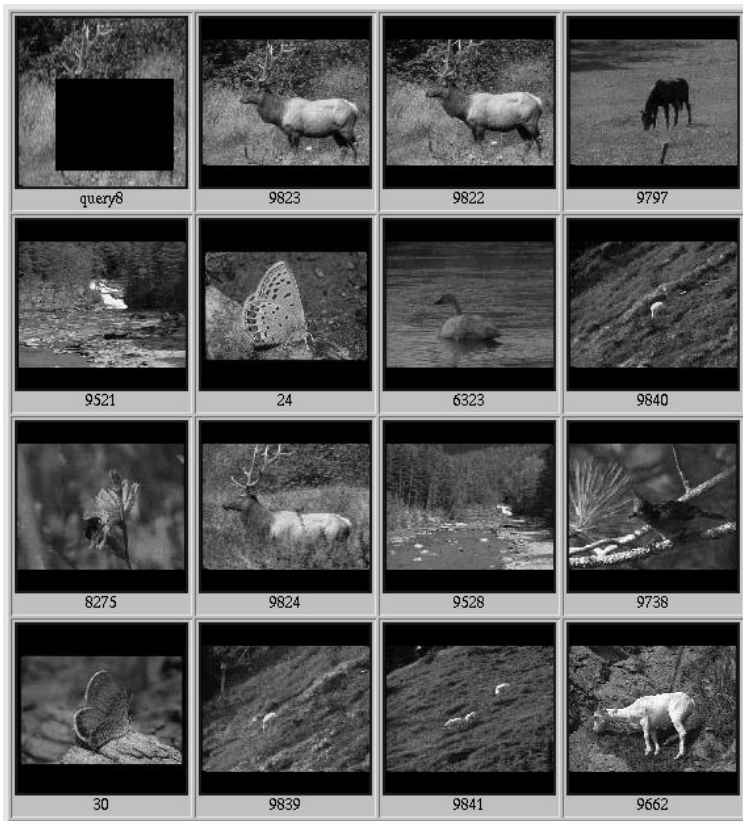
Fig. 13. Partial sketch queries in different resolutions. The upper-left corner image in each block of images is the query. Black areas in a query image represent non-specified areas. Results were obtained from a database of approximately 10 000 images
