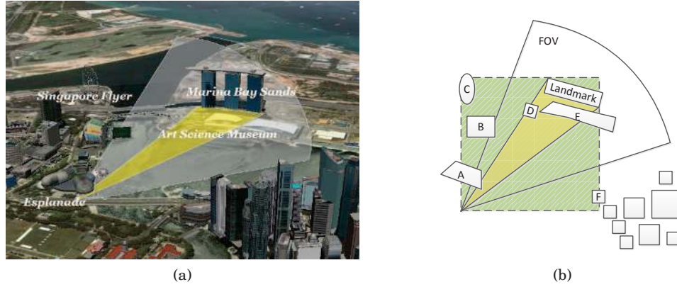
Fig. 2: (a) An illustration of a camera's field of view in Google Earth. (b) The corresponding scene projection on the 2D plane.
