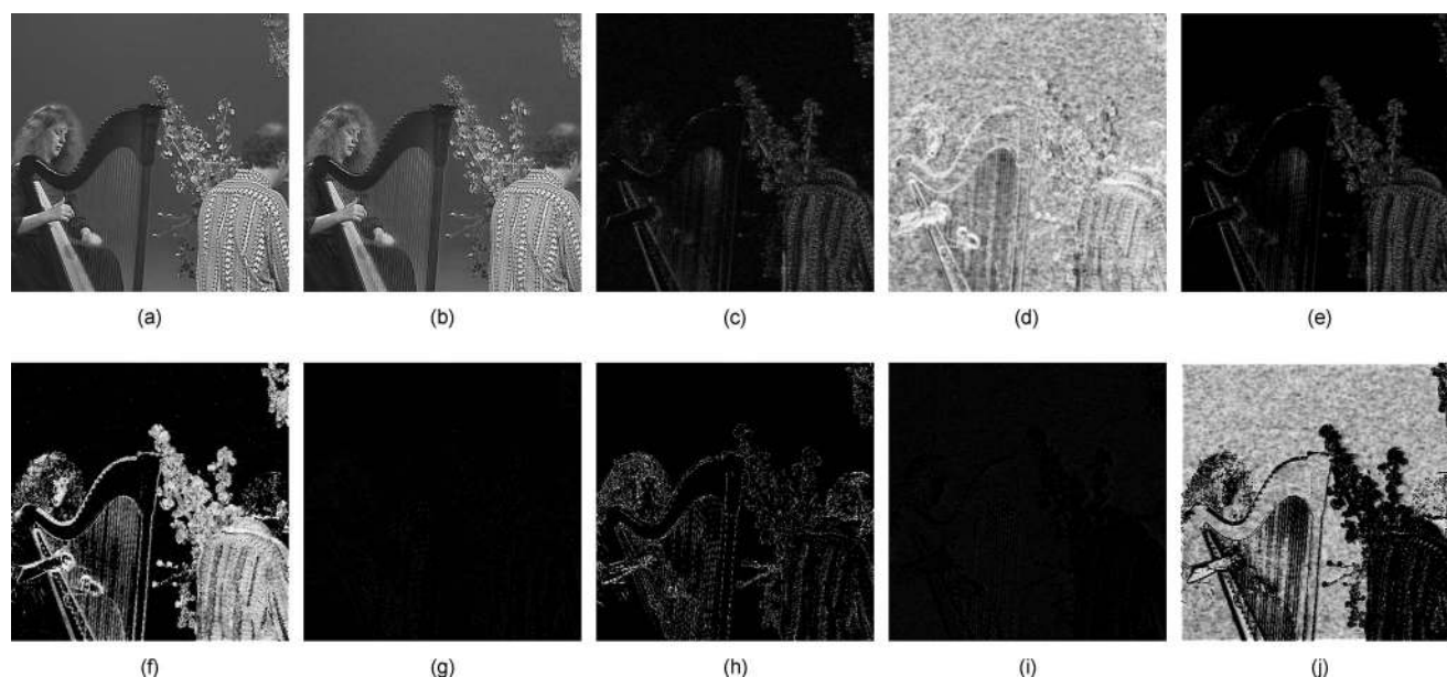
Fig. 2 Illustration of quality maps: (a) original image, (b) distorted image, (c) absolute error map, (d) SSIM index map, (e) absolute error map for edge regions, (f) SSIM index map for edge regions, (g) absolute error map for texture regions, (h) SSIM index map for texture regions, (i) absolute error map for smooth regions, and (j) SSIM index map for smooth regions.
