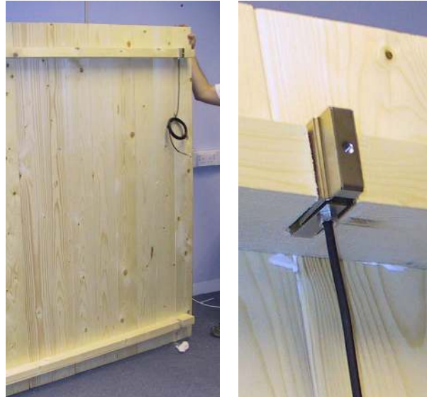
Fig. 4. The floor when it was installed in upright position (left). Enlarged view of the load cell embedded into the floor (right).
