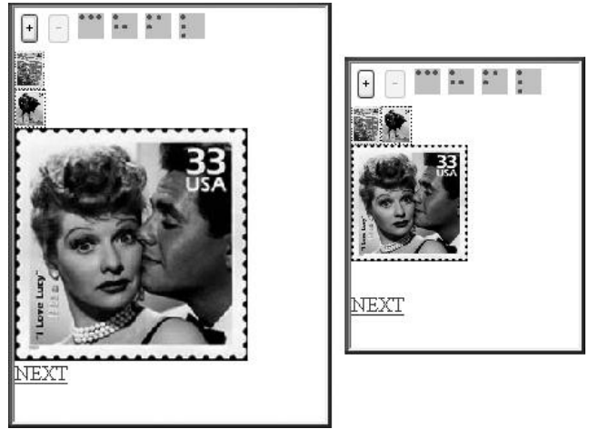
Figure 4: Screenshots of page layout prototype on simulated displays of PDA (shown left) and SmartPhone (shown right). The toolbar at the top of the web page allows the user to manipulate the dimensions and layout of images.
