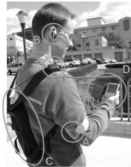
Fig. 5. Wearable Platform for current SenSay prototype: (A) SenseWear armband, (B) BlueSpooon headset, (C) backpack encompassing Life-Book P-1120 with 802.11b transceiver, (D) Tungsten W smart phone, and (E) external antenna for GPS receiver. The SenseWear armband is worn in contact with the skin and normally hidden from view.
