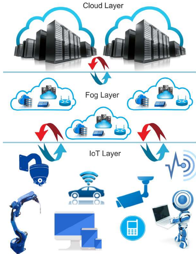
FIGURE 1. Three layered architecture of Fog-based IoT (Flot).
