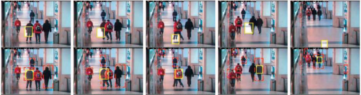
Fig. 14. Frames 40, 56, 68, 135, and 425 of three past shop , 425 frames. (Top) The torso tracker. (Bottom) The CAT tracker.
