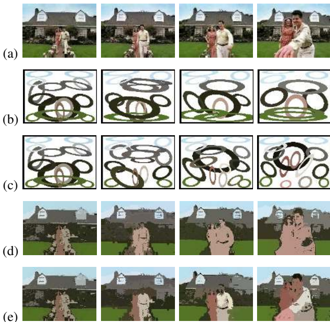
Fig. 3. Video sequence, example 2: (a) selected frames (1,11,21,31) from original sequence; (b) ML model learned per frame, previous frame is used for initialization ( \beta = 0 ); (c) MAP-EM model based on adaptation from previous frame ( \beta = 0.2 ); (d) segmentation maps using the previous frame for initialization (ML); (e) segmentation maps using the MAP-EM estimation.
