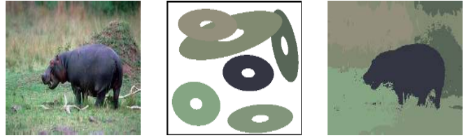
Fig. 1. Input image (left). Image modeling via a mixture of Gaussians (center). Image segmentation using the learned model (right).
