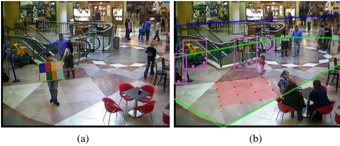
Fig. 1: (a) Detected chessboard points for camera calibration; (b) Horizontal vanishing line (blue), ground plane's projection area (green), ground points (red) to calculate scale factors and reprojection errors, and objects of interest (purple).
