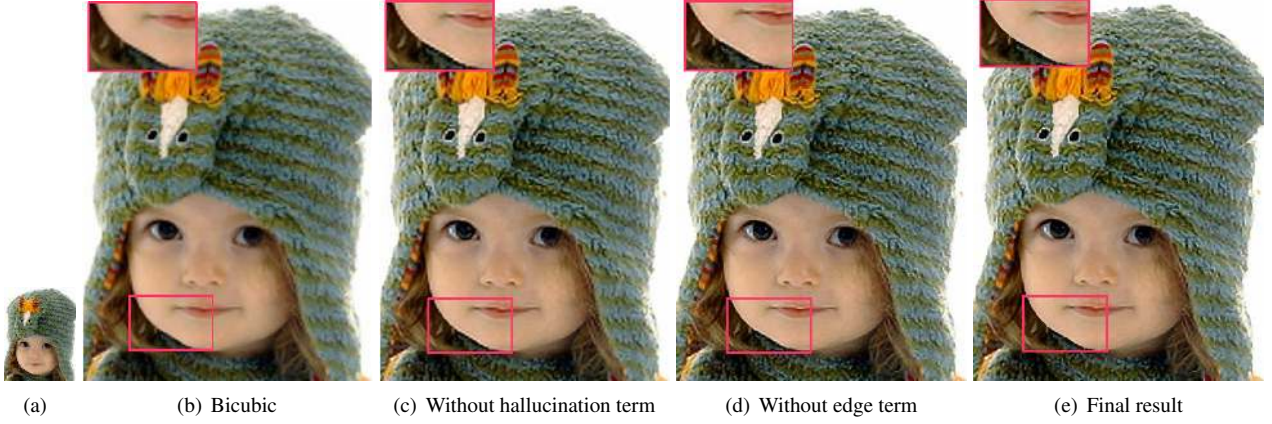
Figure 4. Comparison of super-resolution results ( \times 4 ). (b) shows the result of bicubic interpolation, and it is blurry both in textural regions and along edges. Combining the edge smoothness term and reconstruction term, the result shown in (c) is still not sharp in the hat region, and artifacts along edges are introduced by the reconstruction term. Combining the hallucination term and reconstruction term, the result shown in (d) is sharp in the hat region. However, there are still artifacts along the salient edges. The model combining reconstruction term, hallucination term and edge smoothness term produces sharp edges with minimum artifacts and reasonable textures as shown in (e).
