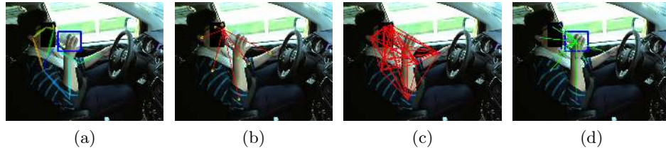
Fig. 2: Contextual descriptors capturing body pose and body-objects interactions: a) detected body joints and cup as an object of interest, b) pairwise relations between nose and the rest of the body joints, c) all possible pairwise relations between detected body joints, and d) pairwise relations between detected cup and various body joints.
