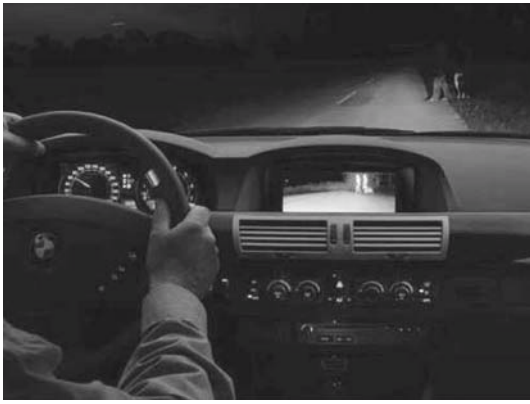
Fig. 1 The BMW night vision system on a vehicle (courtesy of BMW)
