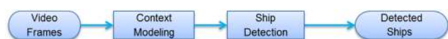
Fig. 3 Framework B: ship detection with sequential processing of context modeling and ship detection.
