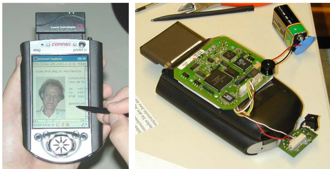
FIG. 3.1. Combining of WLAN and RFID Capabilities in a Commercial PDA
