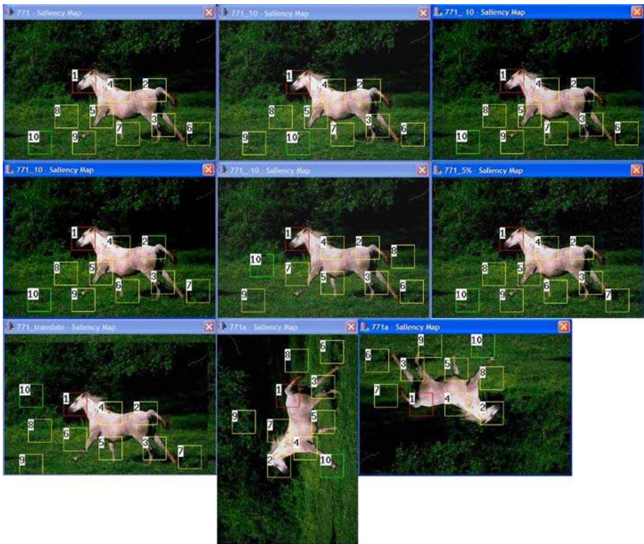
Fig. 12 An example of information path changing due to image alterations: (1,1) Original image ; (1,2) Brighten 10% ; (1,3) Darken 10% ; (2,1) More Contrast 10% ; (2,2) Less Contrast 10% ; (2,3) Noise Adding 5% ; (3,1) Horizontal Shifting 15% ; (3,2) Rotate 90 ; (3,3) Flip 180
