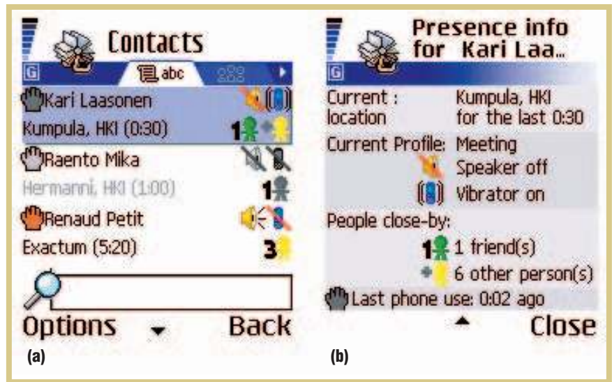
Figure 3. The ContextContacts context representation. (a) ContextContacts replaces the Smartphone Contacts list with one that includes information on current and past location, phone use activity (indicated by hand color), people present, and phone alarm profile. (b) By clicking on the contact in the list, the user sees more details and an explanation of the system's shorthand and icons.
