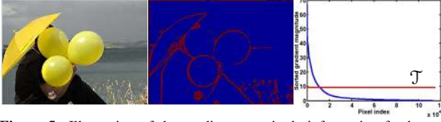
Figure 5: Illustration of the gradient magnitude information for hyperedge saliency evaluation. The left subfigure shows the original image, and the middle subfigure displays the gradient magnitude map I_g^* obtained by binarizing I_g using the adaptive threshold \mathcal{T} , as illustrated in the right subfigure.
