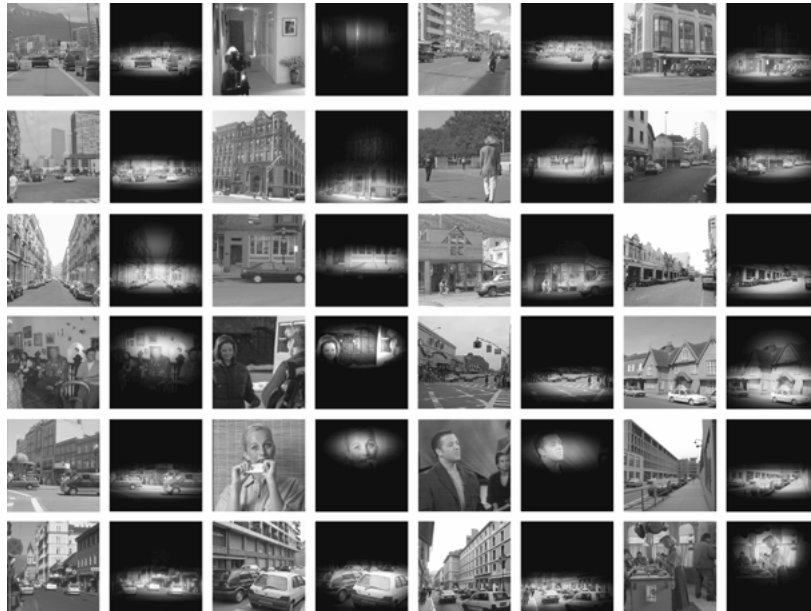
Figure 14. Focus of attention based on global context configuration. Each pair shows the original image and the image multiplied by the function P(\mathbf{x} | \mathbf{v}_C, o = heads) to illustrate the primed regions.
