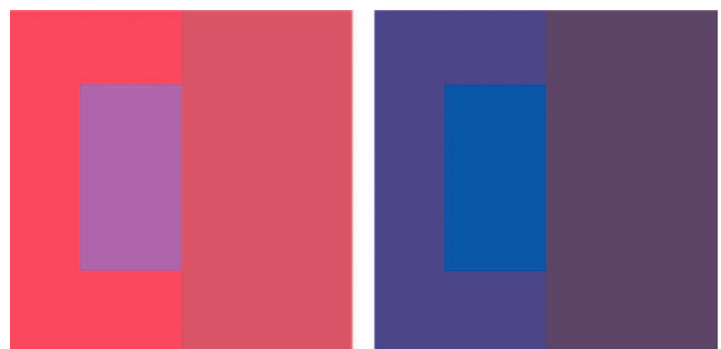
Fig. 15 Visualization of artifacts caused by contour loss: MinDE3D (left) and HPMInDE (right). The left half of a square shows the original colors and the right half shows mapped colors.
