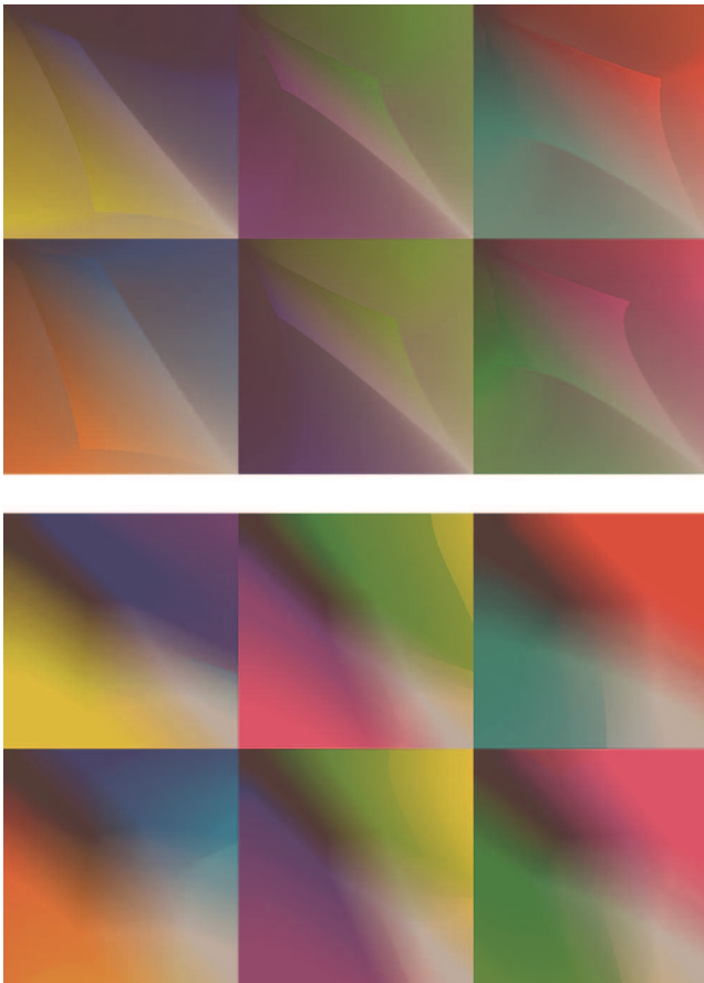
Fig. 11 Artifacts in color gradients: GCUSP1 algorithm showing visible boundaries of regions with different mapping strategies (top), and minimum distance mapping to polygonal approximations of concave gamut border (bottom).
