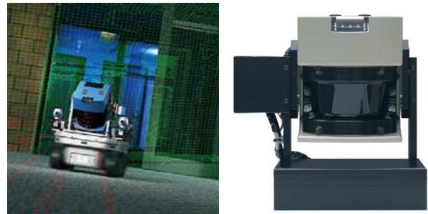
Fig. 1. The KURT3D robot (left) and the IAIS 3D laser scanner (right).
