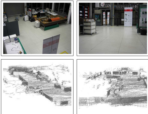
Fig. 9. 3D model of an example scenario. The model was obtained by matching generated 3D point clouds. The robot's trajectory is depicted in Fig. 7.
