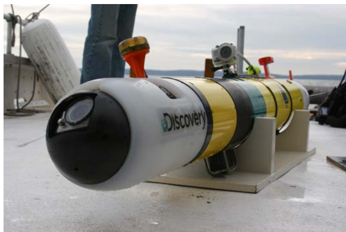
Figure 3. Vehicle equipped with Go-Pro HD video cameras, acoustic navigation system and environmental sensors. ©Big Wave Productions
